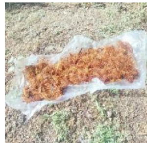
Fig. 3.2 Drying of treated coir
